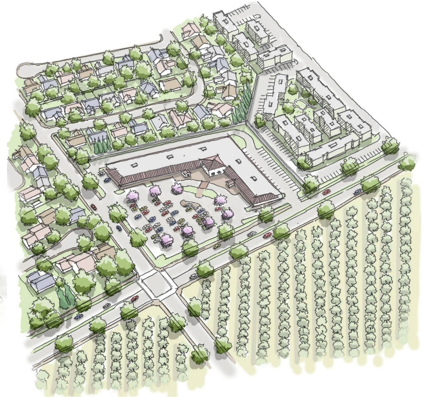
Above right: Example of a Neighborhood Center that is inconsistent with the General Plan, with walls separating homes from destinations; cul-de-sacs and other barriers to transportation connectivity; buildings that set far back from the site frontage; a large amount of parking in front that presents a barrier for pedestrians, bicyclists, and transit; and a location adjacent to agricultural areas instead of centrally located, and convenient to the neighborhood it serves.
